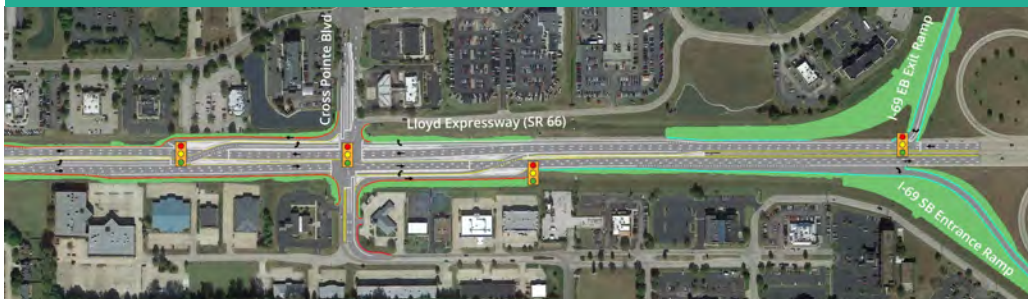
Displaced left turns, New I-69 Signal
