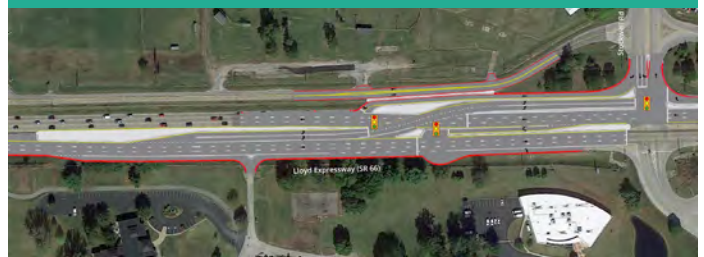
Displaced left turn with boulevard u-turn
