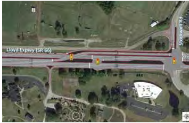
Hybrid solution with EB displaced left turn and WB boulevard left turn
