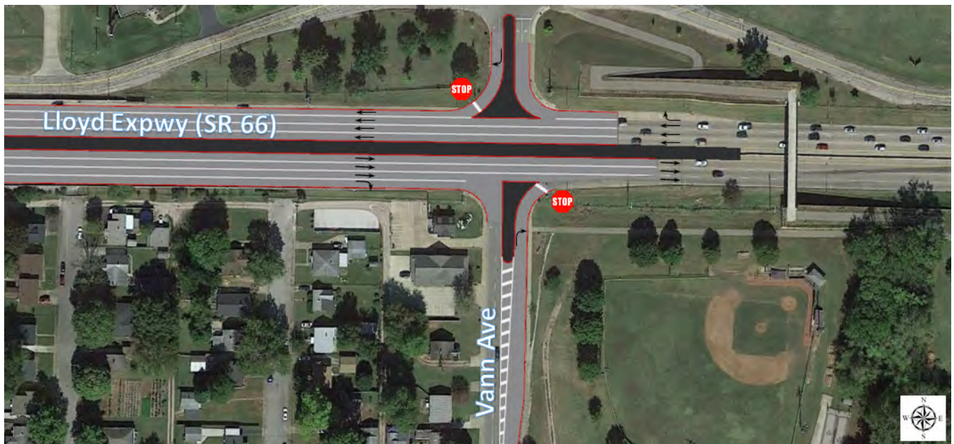
Right-in, right-out (restricted turn movements)
