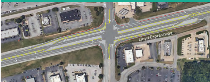
Dual Displaced Left Turns
