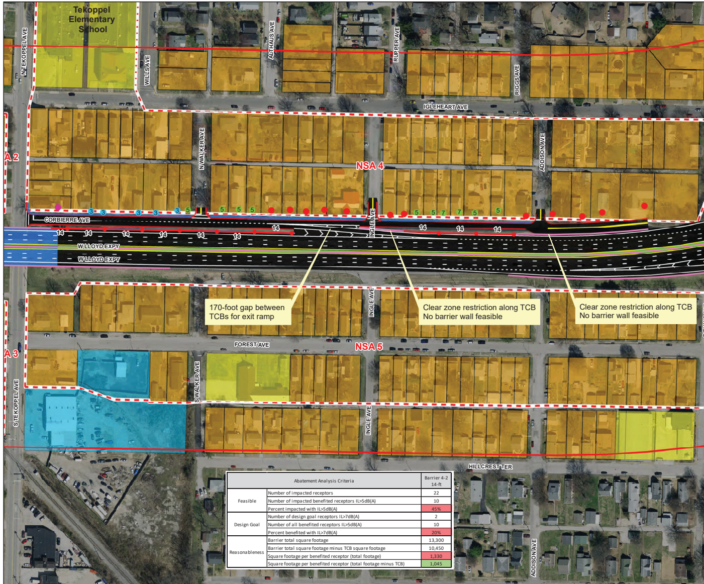
Figure 4B 2040 Design Year NSA 4 Barrier 4-2
