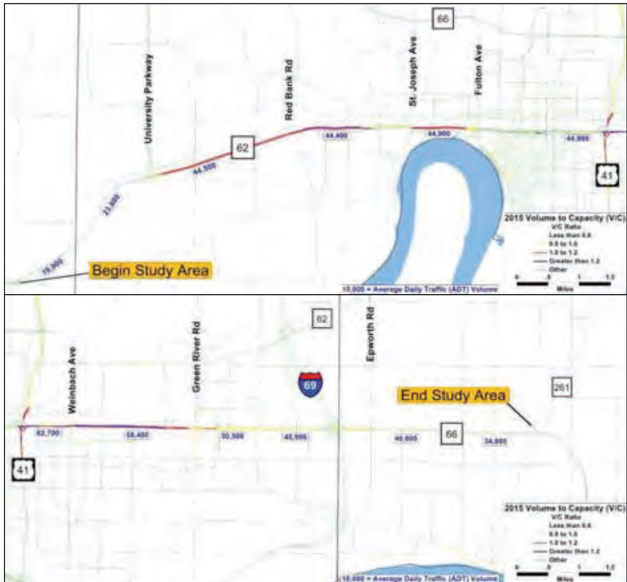
Figure 2.10 Latest Average Daily Traffic (ADT) Counts and Volume to Capacity (V/C) Ratios
